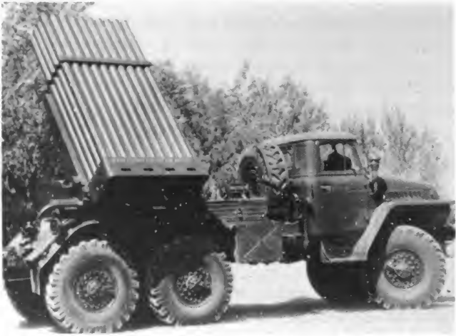
Figure 6-28. Multiple rocket launchers. The 122-mm BM-21, shown here mounted on a URAL-375 truck, has 40 tubes. Mass rocket fires play an important part in the Soviet doctrine of heavy firepower.
